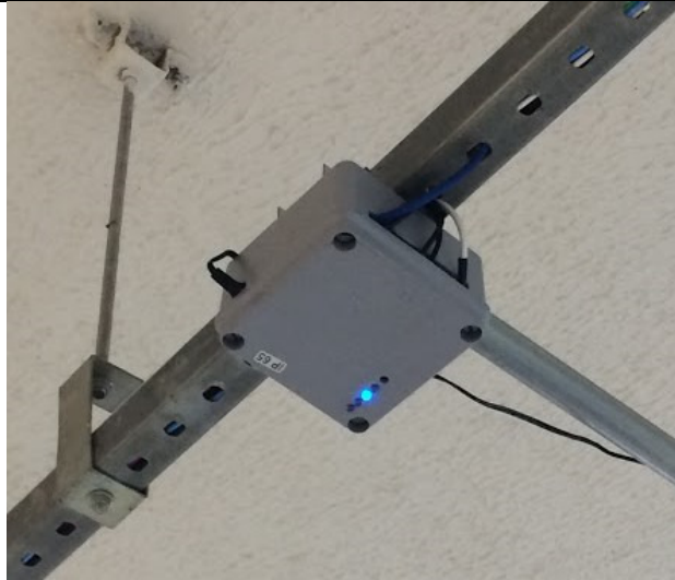
Figure 19. Final prototype in operation installed on an electrical track on the laboratory ceiling
