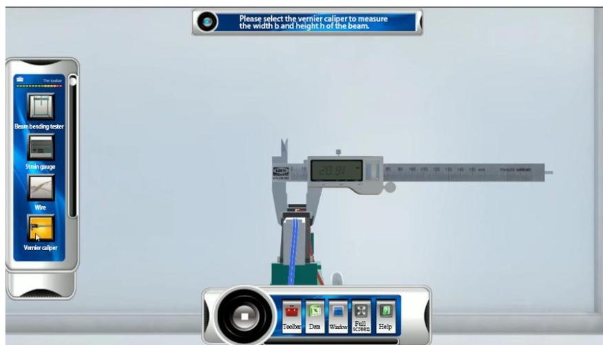
(b) Size measurement of beam
