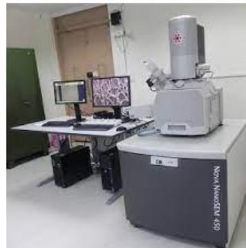
Fig.2. SEM set up [5]
