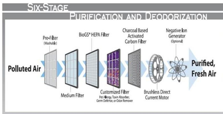
Fig 2.9 Design of Integrated Air purifier for Vehicle/homes
