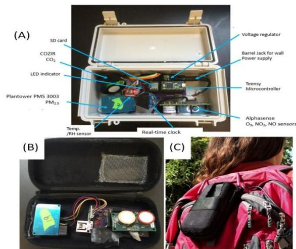
Fig 2.12. (a) All sensor package components in indoor/outdoor sampling case, (b) Personal monitoring case with internal components, and (c) Personal monitor hanging on a backpack.
