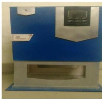
**Fig 2.5** Air purifier using HEPA filter
