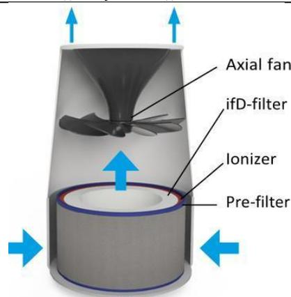
**Fig 2.4** Easy handling air purifier
