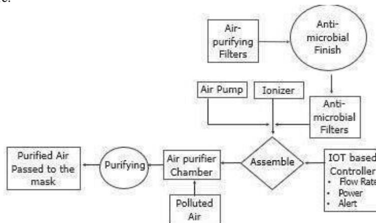
**Fig 2.3** Flow chart for Advanced Air Purifier Facial mask
