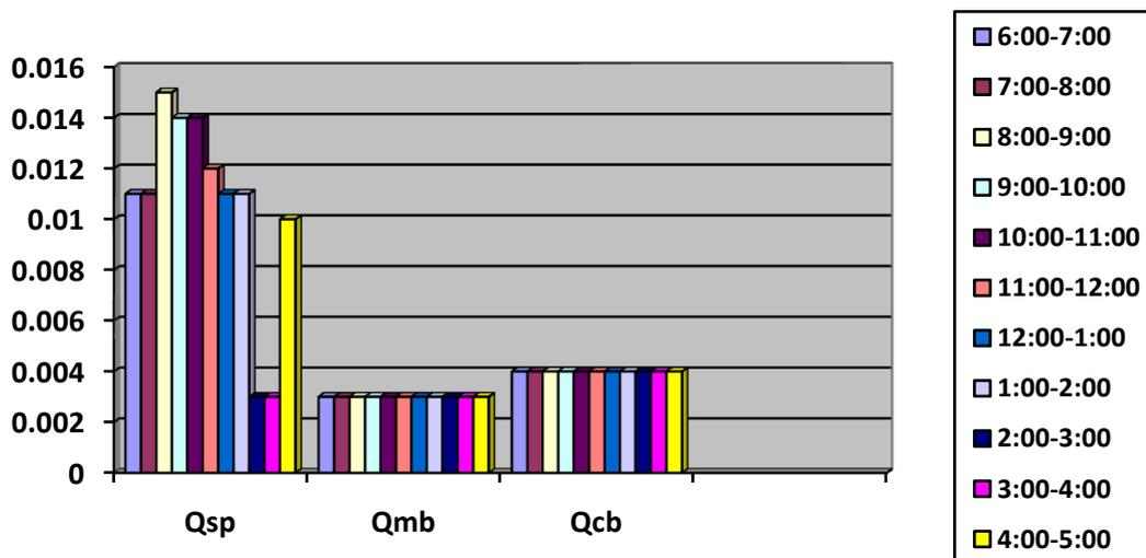
Fig. 5. Discharge performance of solar sprayer powered by the solar panel (Qsp), 1SMF battery (Qcb), and MF9-B battery (Qmb)
