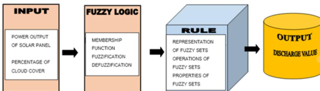
Fig. 4. Diagram of estimating the discharge value at a certain percentage of cloud cover using fuzzy logic
