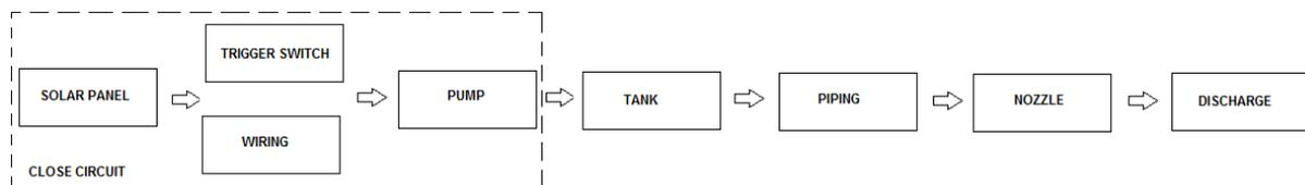
Fig. 2. Operation Diagram
