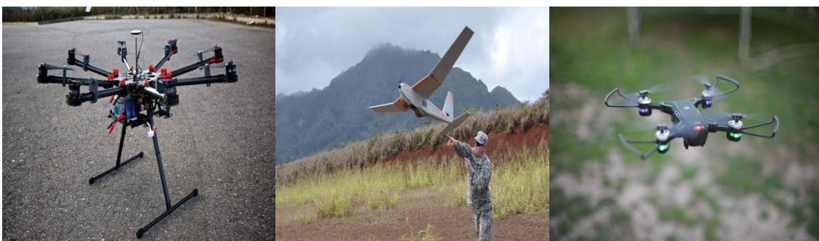
Figure 5.G –Large Drones Figure 5.H –Very Close-Range Figure 5.I – Close Range
