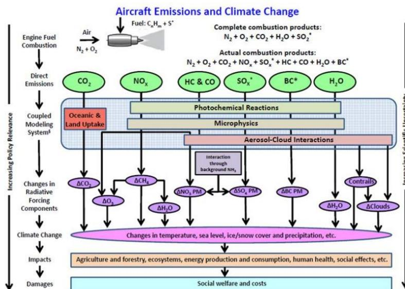
Figure 1: Schematic representation of emissions from aircraft combustion
