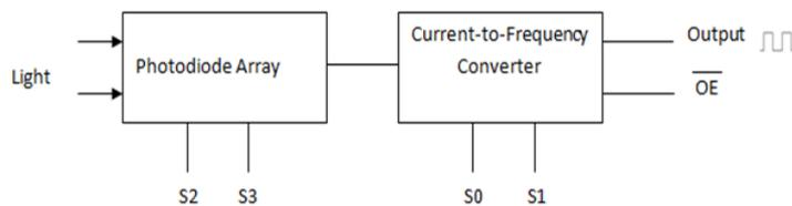
Fig. 2 Light-to-frequency converter
