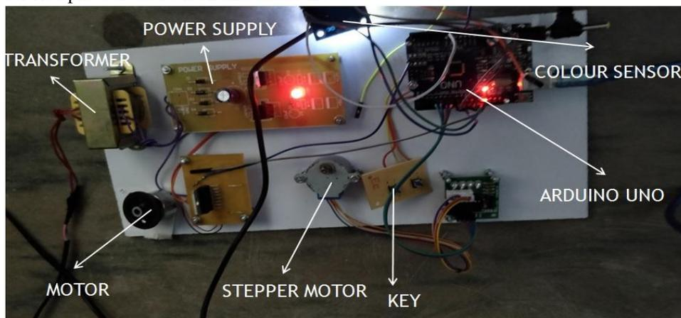
Fig.3 Snapshot of the Experimental Setup to measure intensity with varying distance
