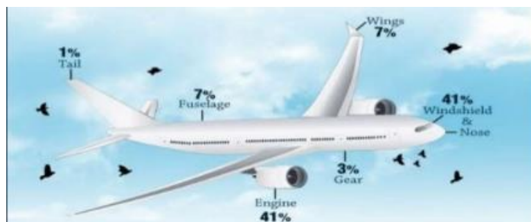
Fig. 1.2: Areas of the aircraft prone to Bird Strike
