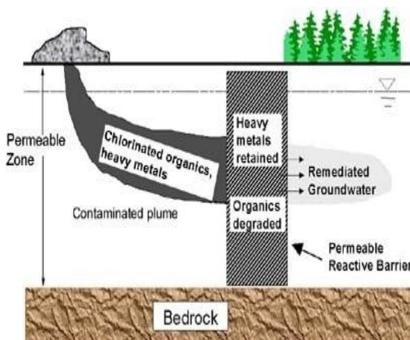
Figure 1.1 Permeable Reactive Barrier
