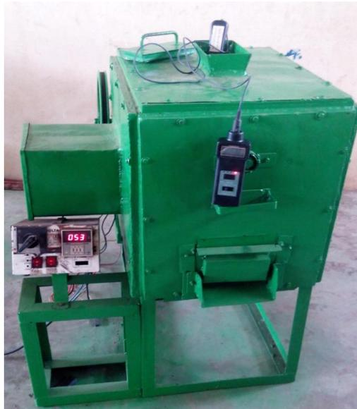
Plate1.5 Moisture meter inserted in the drying chamber for readings.
