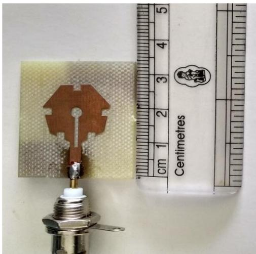
Fig. 16 Fabricated proposed patch Antenna.(Top View )
