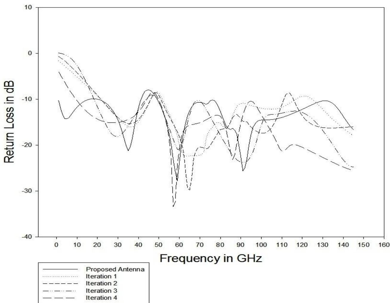
Figure 3: Comparison of Simulated Return Loss(dB) vs Frequency(GHz) of all the iterations
