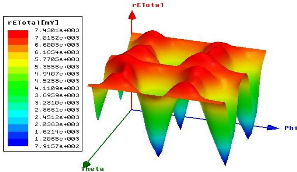
Figure 11 3-D Plot of Simulated Radiation Pattern
