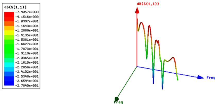
Fig. 7 3-D Plot of Simulated Return Loss vs Frequency.
