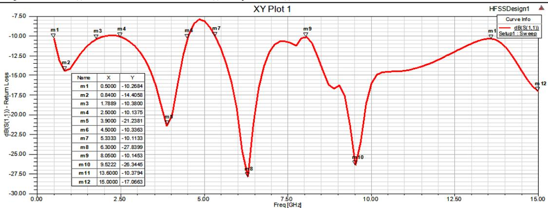
Fig. 6 Plot of Simulated Return Loss(dB) vs Frequency(GHz).
