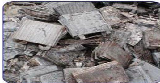
Fig. 3 Scrap of lead acid battery.
