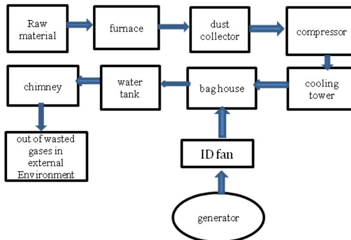
Fig.5 (modified lead recycling plant)
