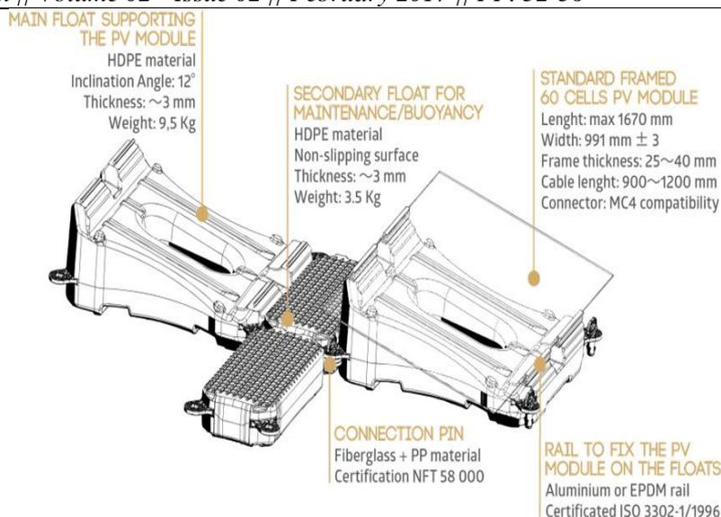
Fig5: Material structural representation
