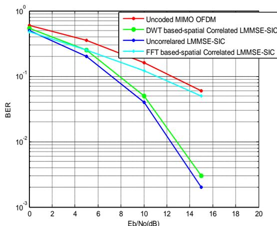
Fig.6 BER vs  $E_b/N_0$  comparison of 2x2 DWT and FFT based LDPC-coded MIMO OFDM system for LMMSE-SIC Demodulator
