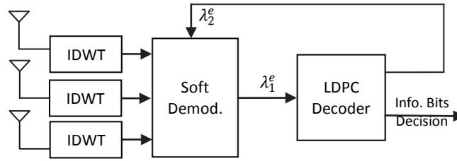
Fig.2 Turbo receiver structure for an LDPC-coded DWT based MIMO OFDM system
