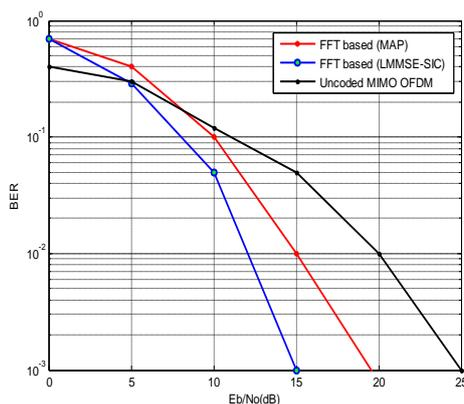
Fig.3 Performance for outage 2x2 LDPC-coded FFT based MIMO OFDM system with no spatial correlation
