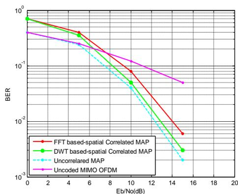
Fig.5 BER vs  $E_b/N_0$  comparison of 2x2 DWT and FFT based LDPC-coded MIMO OFDM system for MAP Demodulator
