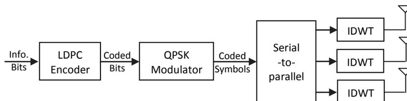
Fig.1 Transmitter Structure of an LDPC coded DWT based MIMO OFDM system
