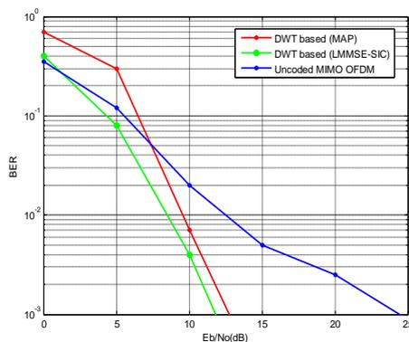
Fig.4 Performance for outage 2x2 LDPC-coded DWT based MIMO OFDM system with no spatial correlation
