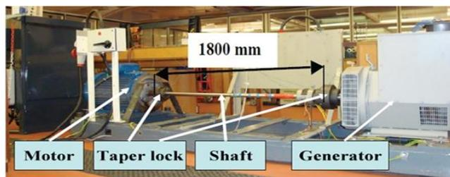
Figure 3.1 Photo of the long shaft rig without shaft cover
