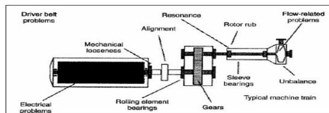
Fig. 2.1 A typical machinery system
