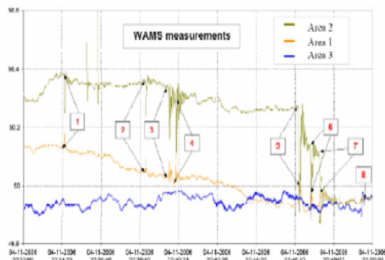
Fig. 5 PMU measurements from three areas during reclosing attempts
