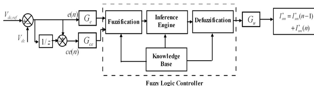
Fig. 2. Detailed structure of fuzzy logic controller
