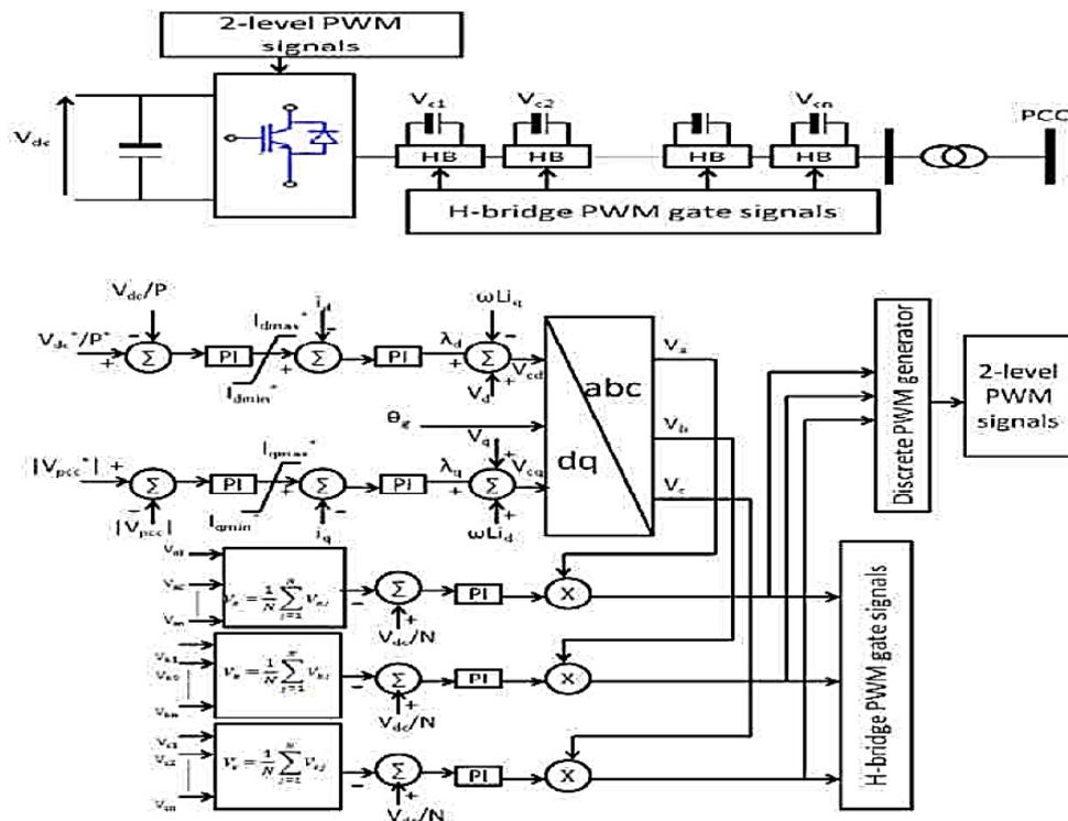
Fig. 4. Schematic diagram represents the control layer of the hybrid multilevel converter with ac side cascaded H-bridge cells
