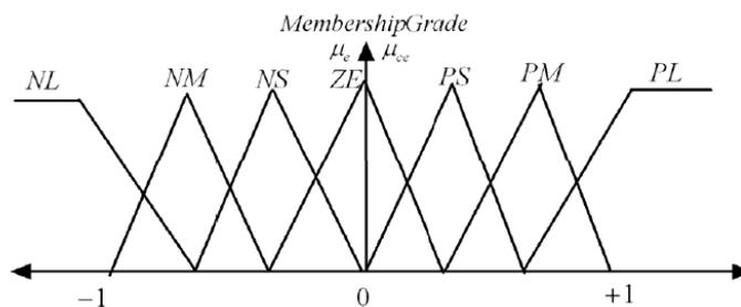
Fig. 3(a) Error 'e' and change in error 'ce'
