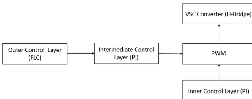
Fig. 5. Block diagram illustrating overview of the control scheme.
