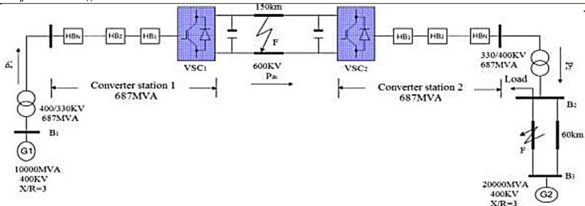
Fig. 6. Proposed HVDC transmission system
