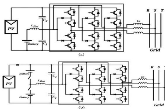
Fig.6. Proposed configurations for integrating solar PV and battery storage: (a) basic configuration; (b) improved configuration.
