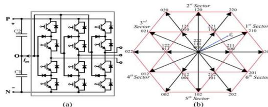
Fig.1. Typical three-level inverter (a) structure of circuit, and (b) three-level inverter space vector diagram for balanced dc-link capacitors [6].
