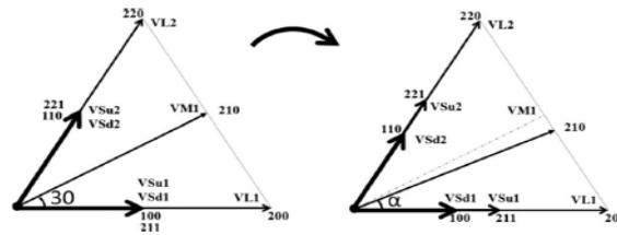
Fig.4. Vector diagram in the first sector of fig.(b) Presenting the change of the vectors using balanced dc and unbalanced dc assuming  $V_{c1} < V_{c2}$ .
