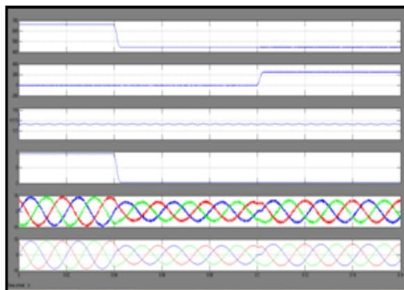
Fig.9. Simulated results for the first scenario. (a) Active power injected to the grid. (b) Reactive power injected to the grid. (c) PV module DC voltage. (d) Battery current. (e) Inverter AC current. (f) Grid current.
