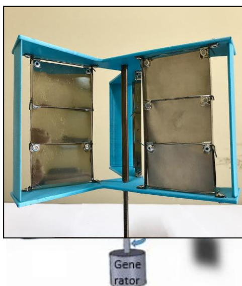
Figure 5 a) Front view for the hybrid WT b) Hybrid WT of vane-type in the middle of the H-rotor
