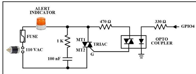
Figure3. Alert indicator electrical interface.
