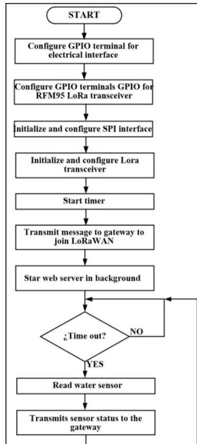
Figure4. Terminal node program flow chart
