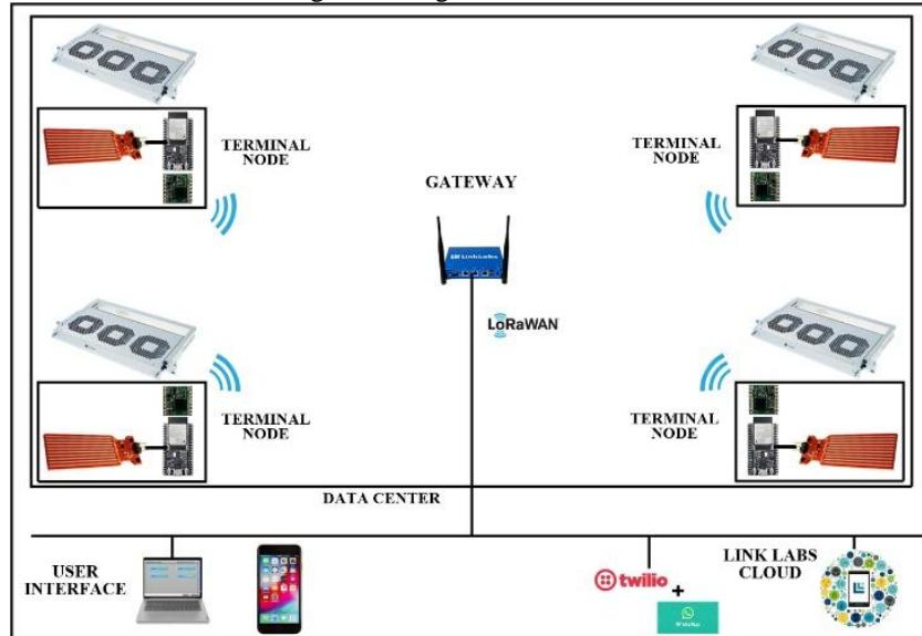
Figure 1. System functional block diagram
