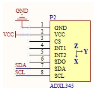
Fig. 2 ADXL345 circuit diagram
