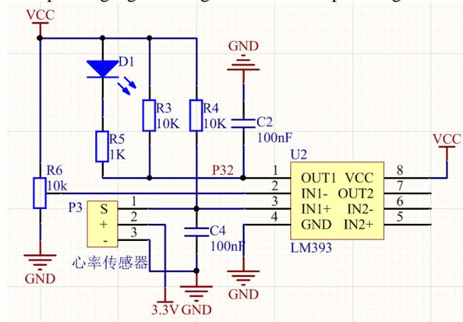
Fig. 4 Heart rate acquisition circuit
