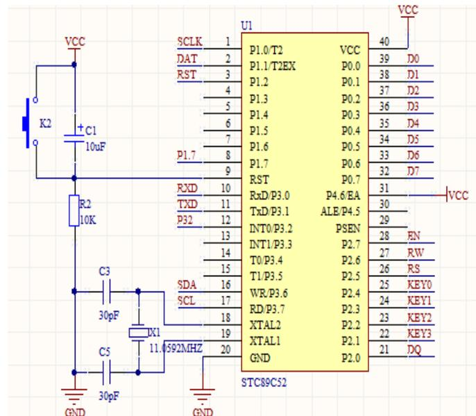
Fig. 1 STC89C52 single-chip microcomputer
