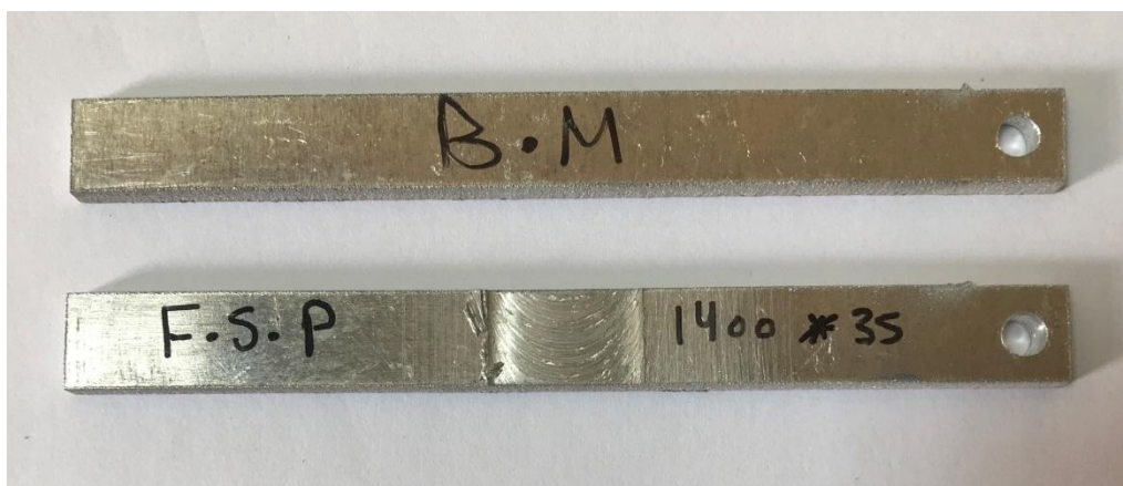
Figure (3): fatigue testing specimens
