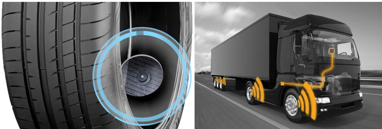
Fig.1. Schematic view of a sensor embedded tire
