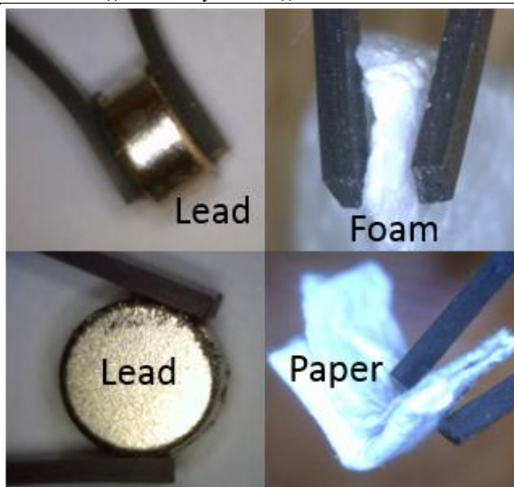
Fig. 4. Microscopic image of gripper's jaws during the holding and maintaining of objects.
