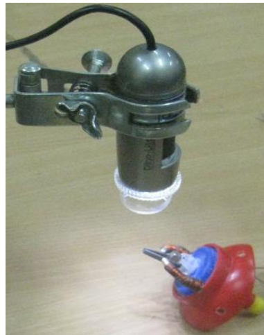
Fig. 7 Microscopic measurement setup of jaw's curvature angle of miniature gripper
