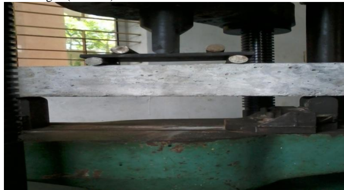
Fig 7. Flexural strength test
