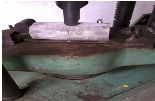
Fig 6: Split Tensile Strength Testing Arrangement
