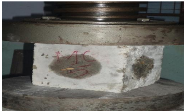
Fig 5: Compressive Strength Testing Arrangement
