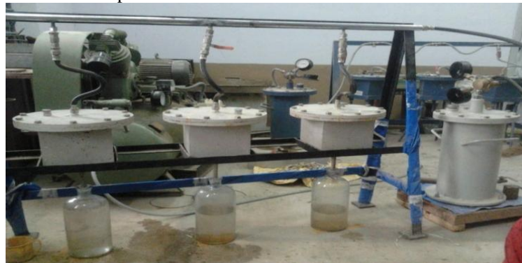
Fig 8: Permeability Testing Arrangement
