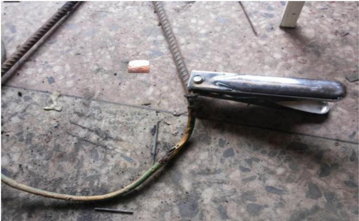
Fig.1 (b): return current cable(earth)
