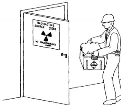
Figure No. 17: A portable gauge is returned to the source store.
