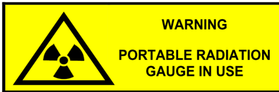
Figure No. 19: Example of a suitable warning sign for posting in the area adjacent to portable density / moisture gauge when in use:
