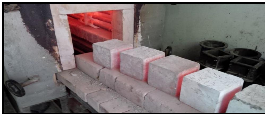
Figure 1: Cubes after Exposing to 800°C in Bogie Hearth Furnace
