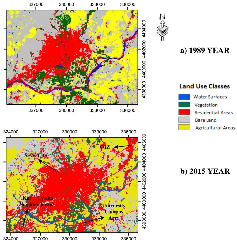
**Figure 3.** Land use distribution data obtained from Landsat-4 TM and Landsat-8 OLI images
