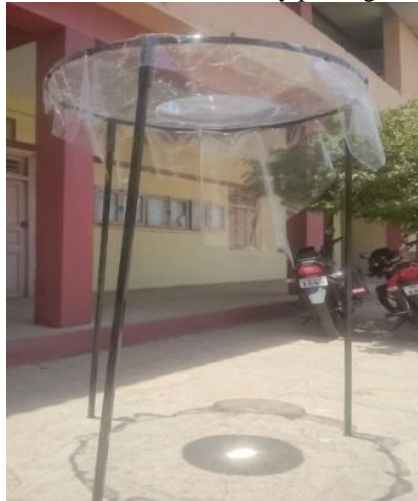
Fig. 1 Experimental set up of solar lens concentrator
