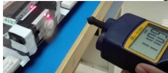
Fig.3. Measuring RPM of Excitation Motor
