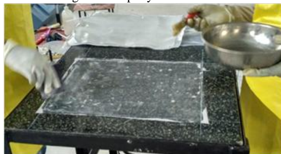
Figure 16: Peel ply on mold surface
