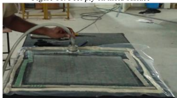
Figure 17: Vacuum bag process
