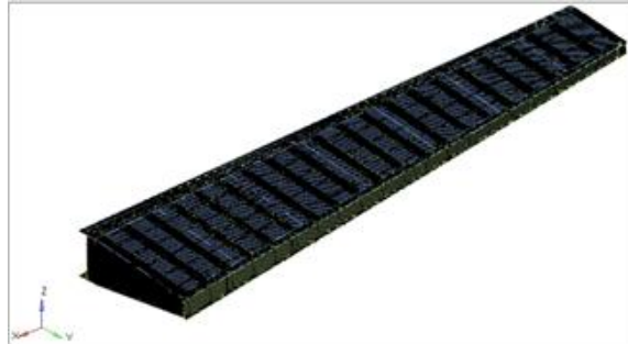
Figure 1 : Finite Element Model of wing
