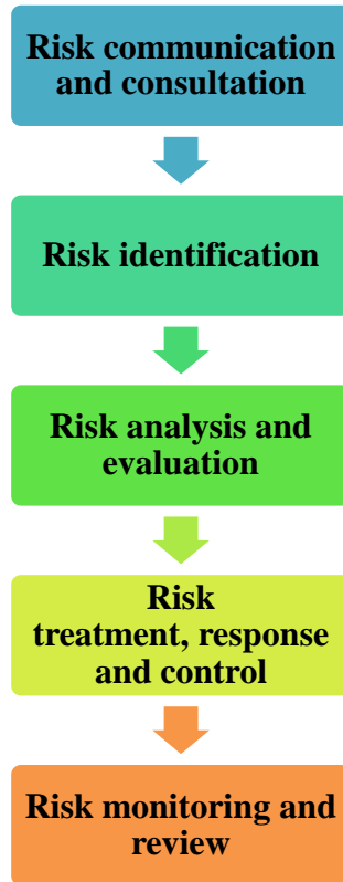
Figure 8. Risk management model for construction projects
