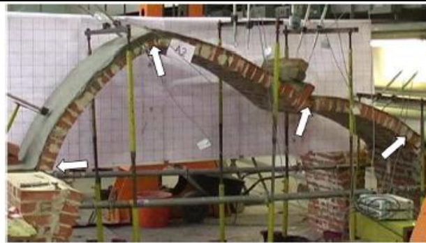
Fig.12. A 2 arch destruction scheme with marked hinging spots (Bednarzet al 2011).
