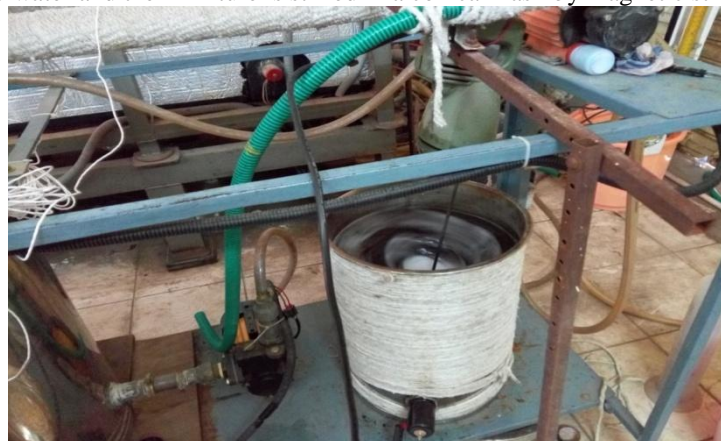
Fig: 2.2: Nano fluid preparation using mechanical stirrer
