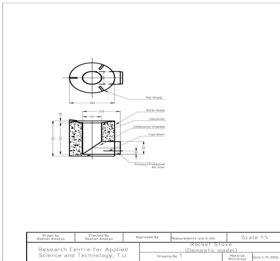
Fig. 3: Diagrammatic Sketch of Rocket Stove (Longitudinal Section)
