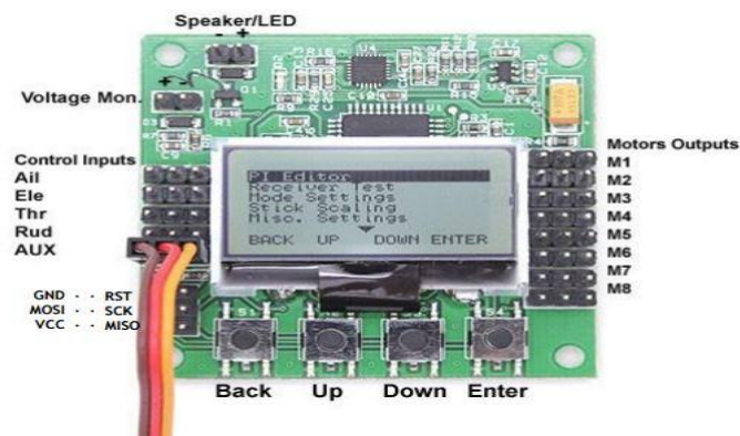
Figure 3: KK Multi rotors Control Board
