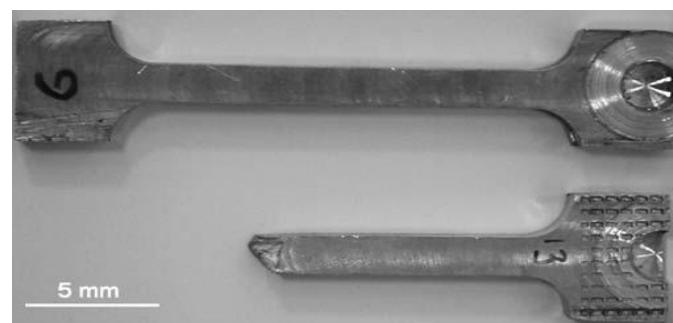
Fig.2. Macrograph of the specimens used for fatigue tests
