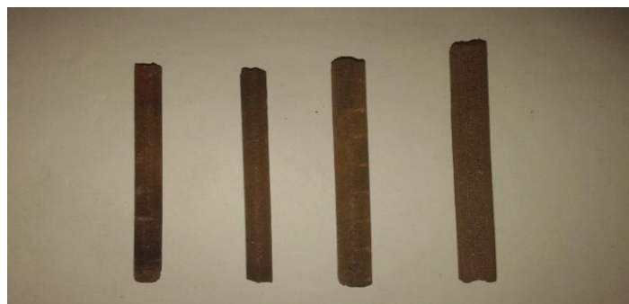
Fig :8 Metallic wicks for different diameter
