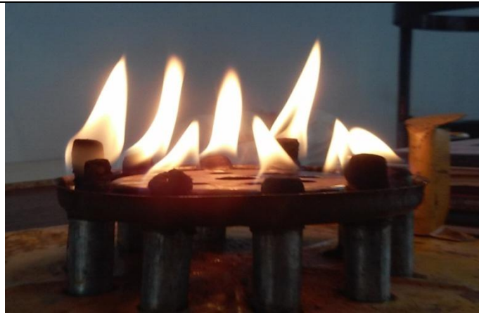
Fig 9 Metallic wick stove with wick burning using Biodiesel(inside)
