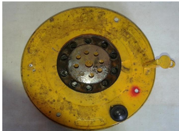
Fig 6: Modified Nutan Stove with Metallic wick (Plan)
