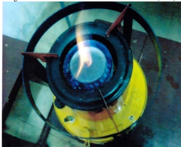
Fig 7 Metallic wick stove with wick burning
