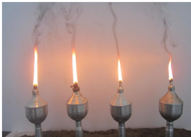
Fig 10: Variation of flame height with different wick diameter
