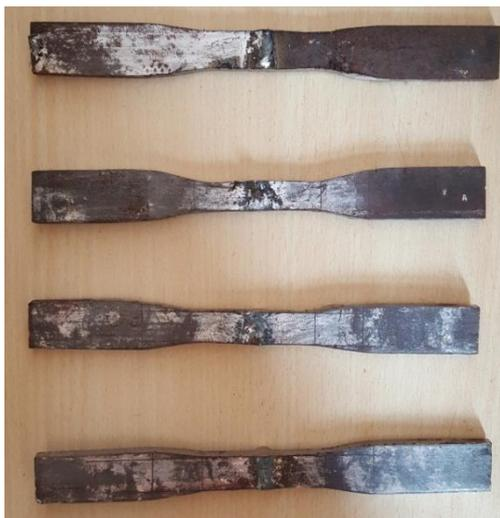
Fig 2.5: 6mm thick tensile specimen
