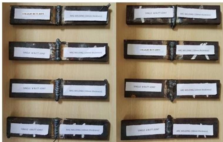
Fig 2.3 MIG and MAW test coupons
