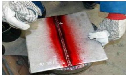
Fig 2.11: Dye penetrant inspection
