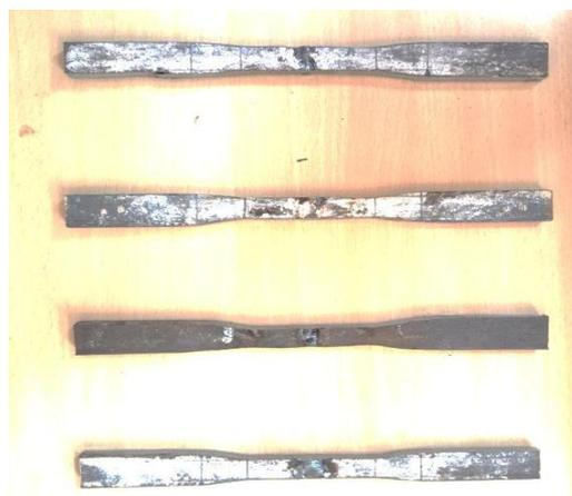
Fig 2.7 10mm thick tensile specimen
