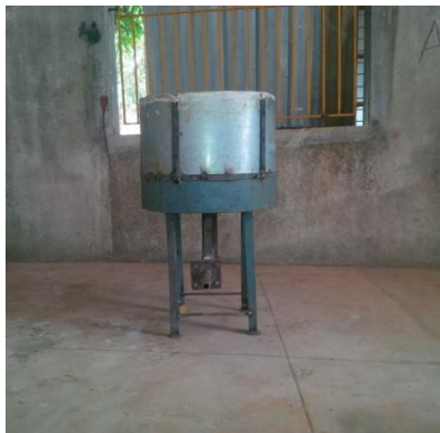
Fig (1) newly fabricated fire brick floor furnace
