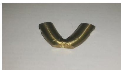
Fig (15) specimen after charpy test
