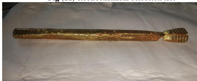
Fig (13) specimen after tensile test
