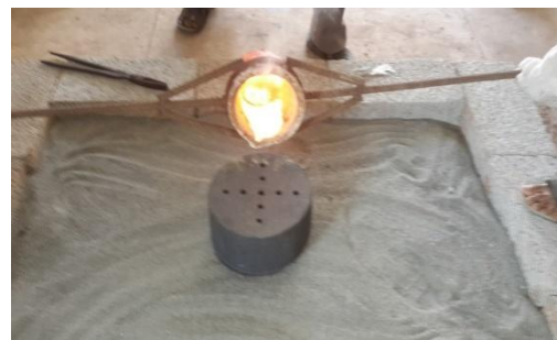
Fig (6) pouring molten metal into the mould cavity
