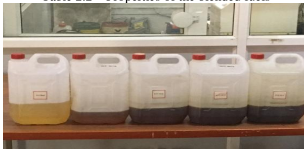
Fig 2.2 – Prepared Blends (B0, B5, B10, B15, B20)
