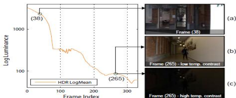
Figure 2: The visual trade-off between emphasizing spatial contrast (a, b) and temporal contrast (a, c). While in both settings frame 38 remains the same (a), frame 265 can be adjusted to either maintain spatial (b) or temporal contrast (c).
