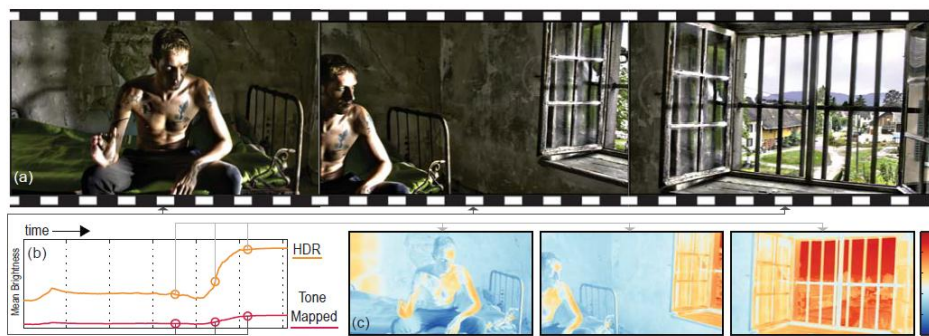
Figure 1: Our method allows local tone mapping of HDR video where the scene illumination varies greatly over time, in this case more than 4 \log_{10} units (c). Note that our method is temporally stable despite the complex motion of both the camera and the actor (b), and the resulting tone mapped video shows strong local contrast (a). The plots show the logmean luminance of the HDR video and the mean pixel values of the tone mapped video.
