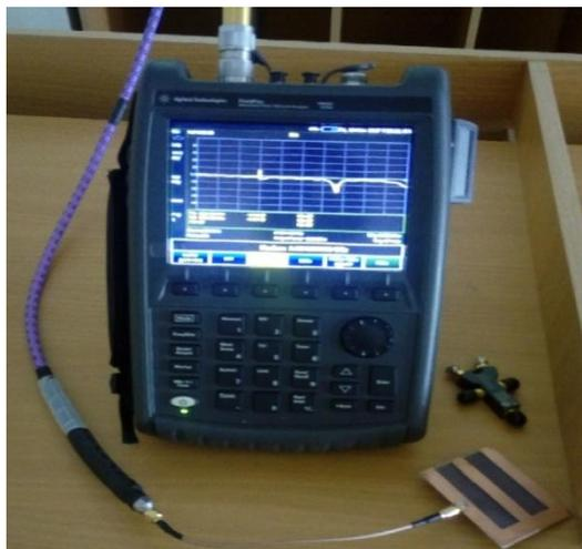
The Screenshot of Microstrip patch antenna parameter measurement using On-field network analyzer.
