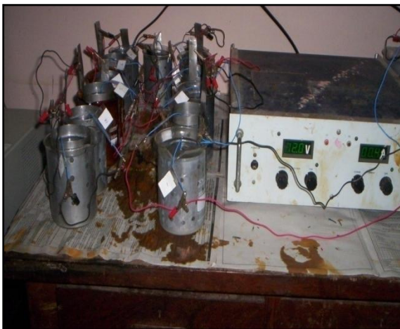
Fig.10 Impressed Voltage Test Setup
