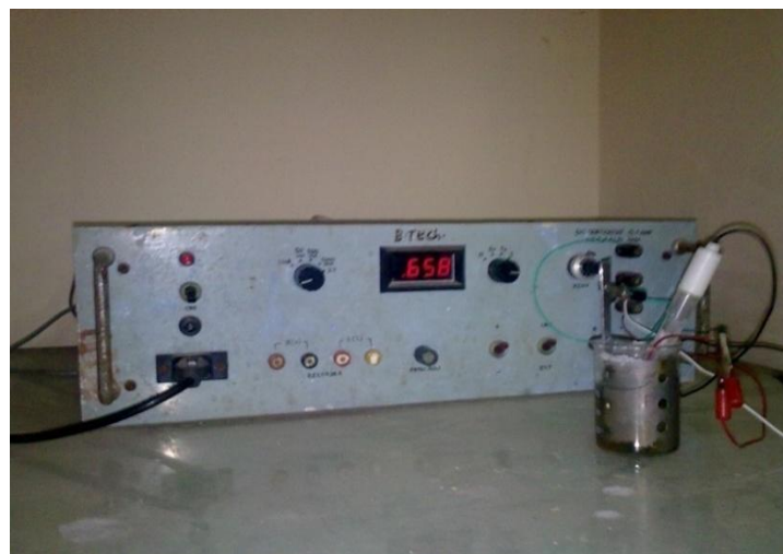
Fig.12 Anodic Polarization Test Setup
