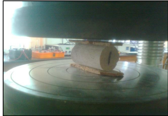
Fig.7 Split Tensile Testing Image
