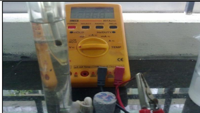
Fig.9 OCP Test Setup
