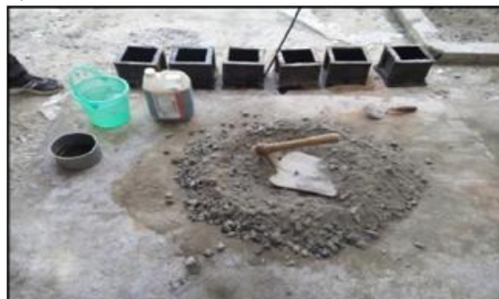
Fig 3(a) Casting of cubes
