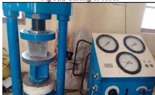
Fig 3(b) Compression testing of cubes
