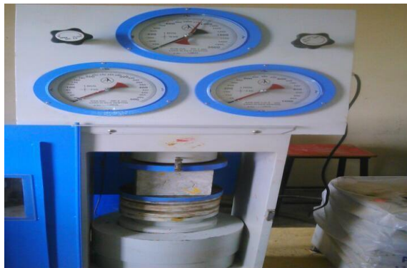
Fig4. Compression strength of concrete cube.
