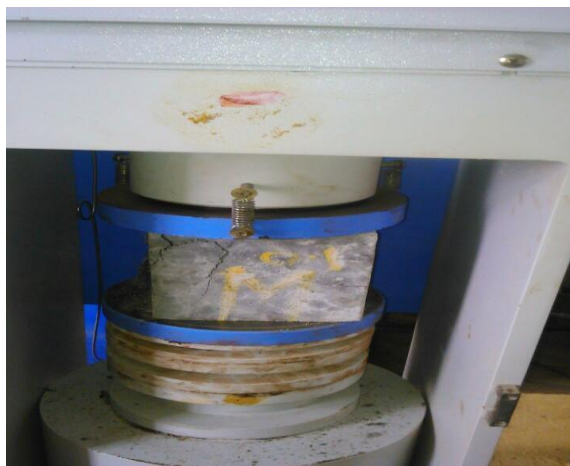
Fig5. Fracture in the concrete cube.
