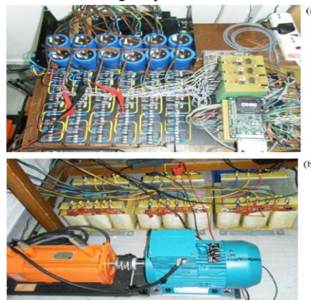
Fig. 17. Hardware implementation: (a) the proposed inverter prototype and (b) phase-shifting transformers, induction motor load, and servo brake system
